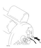
8 Replace reattach green ground wire and grounding nut.
